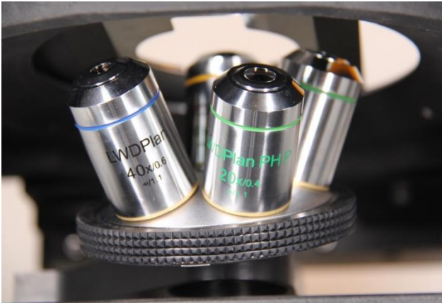
Quintuple Nosepiece, With Positive Click Stops
