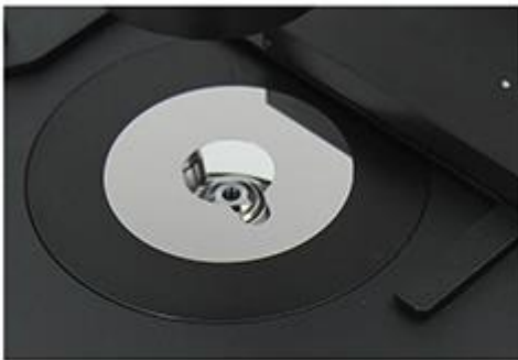
A54.2601-D4 Mechanical Stage Size 210x241mm Round Slide Size \Phi 110mm
