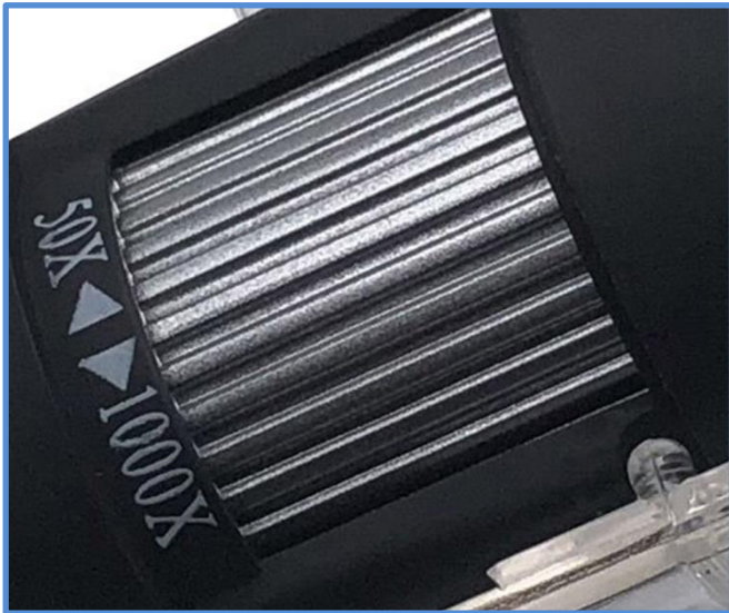
Optical zoom in/out support total magnification 50x-1000x
