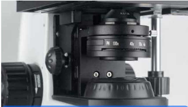
Abbe Condenser With Dark Field & Phase Contrast Interface, Up/Down Adjustable
