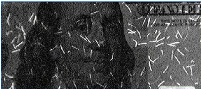
Fluorescent Anti-counterfeiting Mark Excited Filter 580nm Receiving Filter 740nm, Magnification 6x
