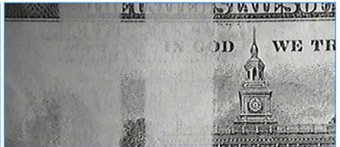
Building Anti-counterfeiting Mark Receiving Filter 700nm, Magnification 2x
