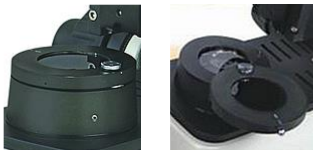
Polarizer, Sliding In/Out of Optical Path, On Top Of Collector
