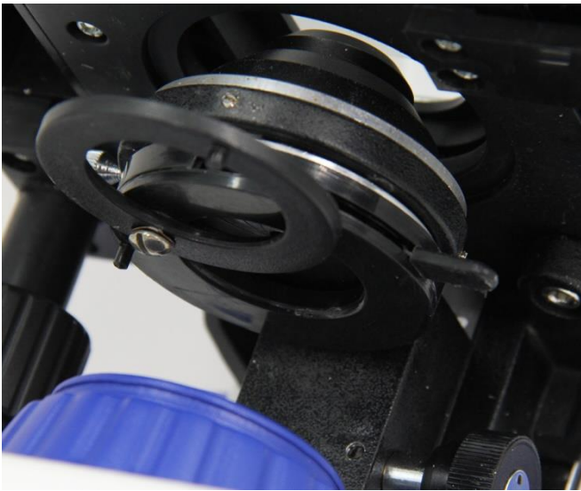
Abbe Condenser N.A.1.25, Rack & Pinion Adjustable
