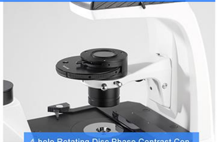
4-hole Rotating Disc Phase Contrast Condenser For Standard To Change Bright Field And Phase Contrast Fast
