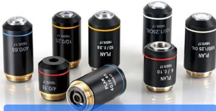
Achromatic & Plan Objective 4x10x 40x100x
