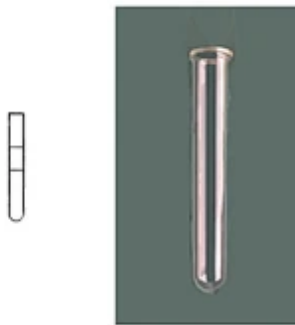
E22.1713 Blood Digestion Tube For Non-Protein Nitrogen Determination
